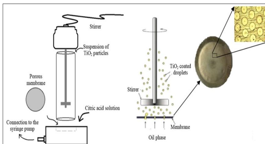
**Figure 2.** Dispersion cell and nickel porous membrane (Gasparini et al., 2008)
