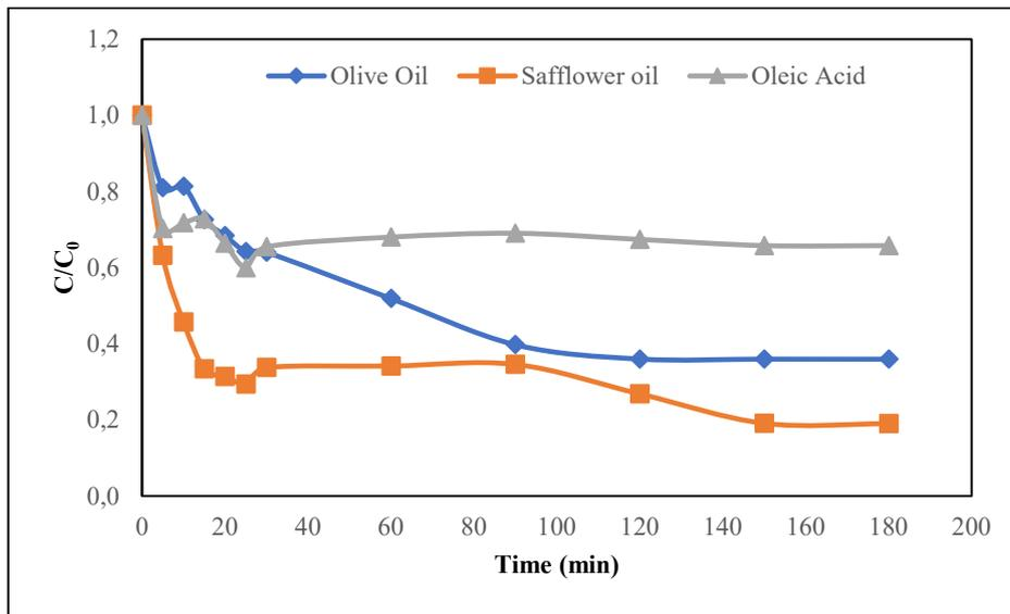
Figure 7. Effect of oil type (Conditions: 0.5 BA-TiO<sub>2</sub> + 2g CA)
