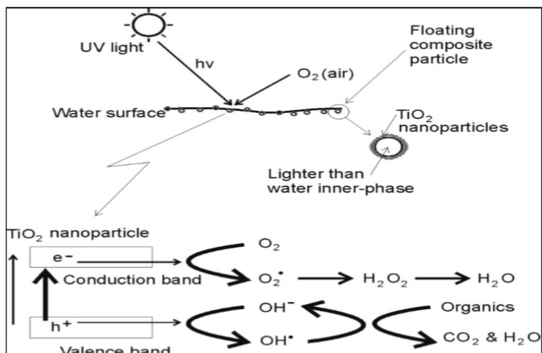
**Figure 1.** Schematic of composite TiO<sub>2</sub> forming free radicals to decompose organic matter (Holdich et al., 2012).
