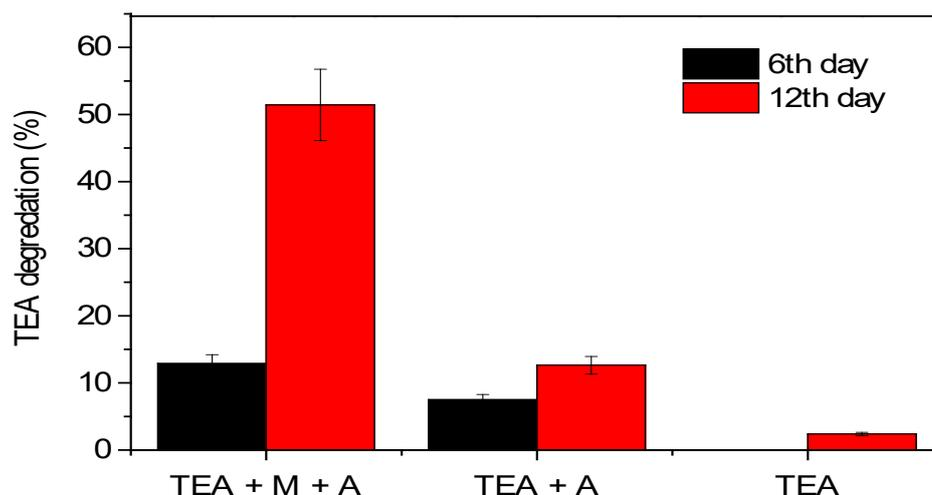
**Figure 4.** Comparison of TEA degradation during microalgae cultivation (M) and aeration (A) compared to blank TEA solution after 6 and 12 days of operation
