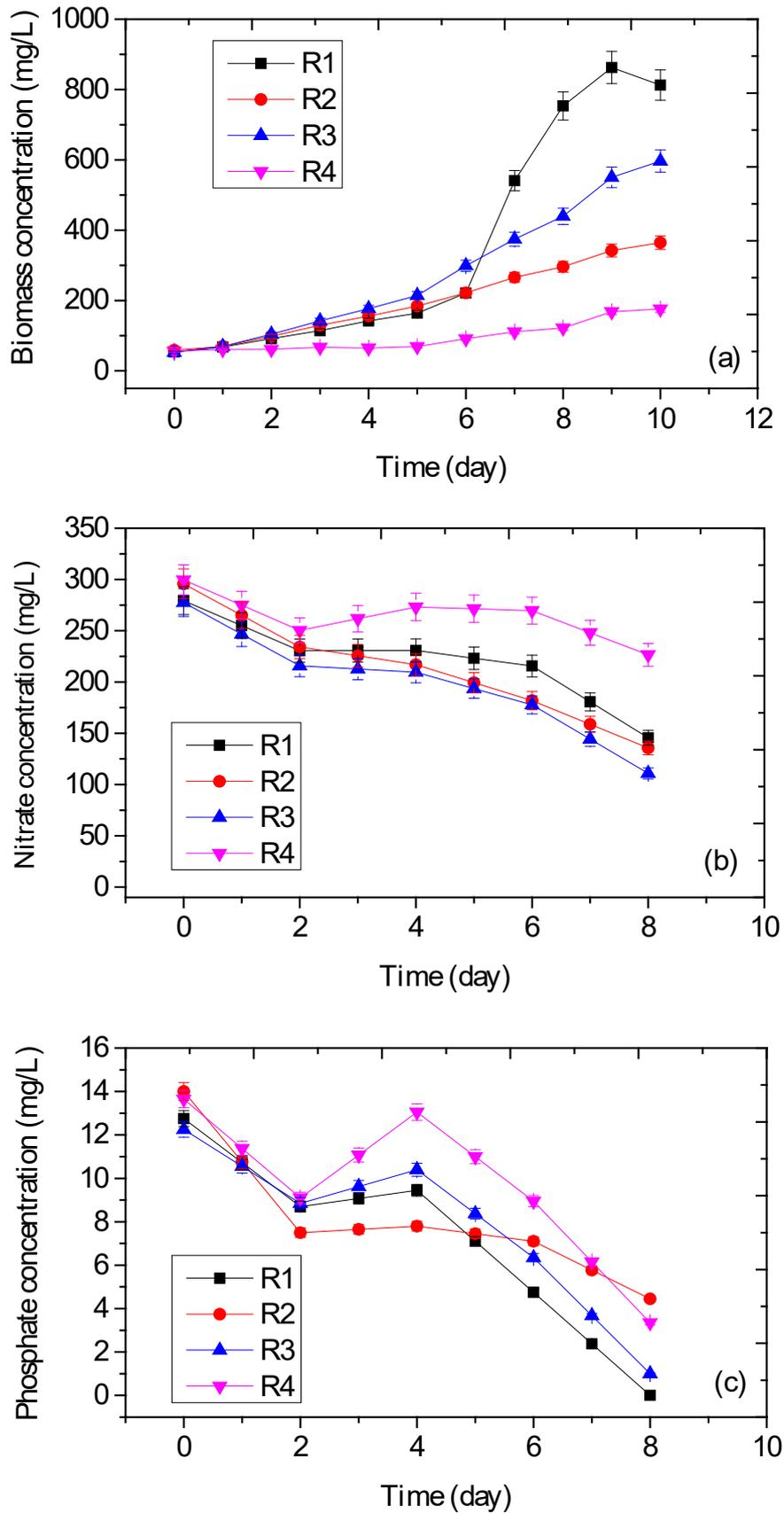
**Figure 5.** Comparison of the cultures grown in different reactors in terms of (a) biomass growth, (b) nitrate, and (3) phosphate consumptions
