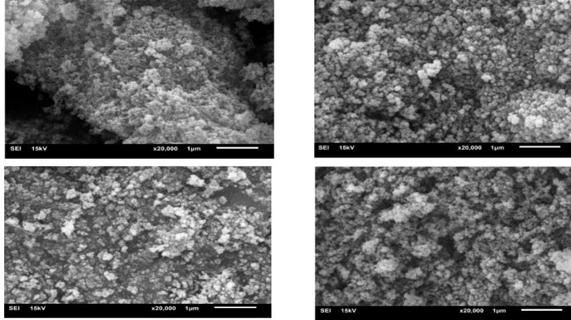
Figure 3. SEM images of (A) BA-TiO<sub>2</sub>, (B) SA-TiO<sub>2</sub>, (C) CA-TiO<sub>2</sub> and (D) pure TiO<sub>2</sub>
