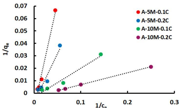
Figure 5. Langmuir isotherms of the hydrogels.
