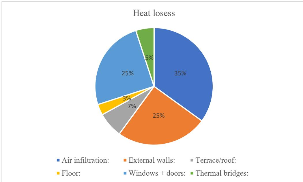
Figure 5. Heat losses from each building element
