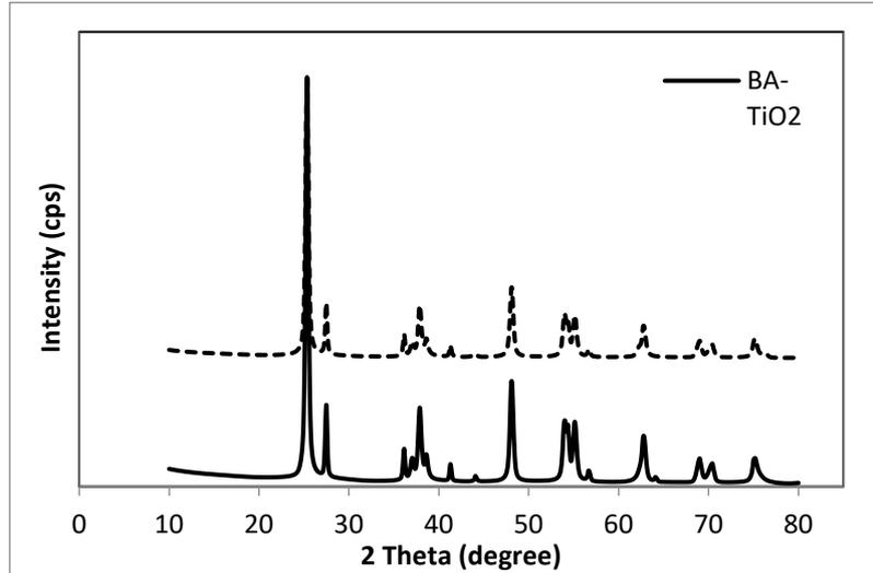
Figure 4. X-Ray diffraction pattern of TiO<sub>2</sub>
