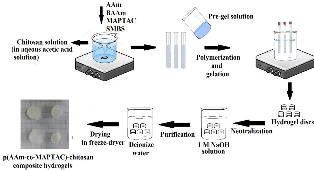
Figure 1. Synthesis schema of the p(AAm-co-MAPTAC)/chitosan hydrogels.
